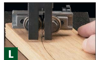
▲ The Powermatic guidepost has a blade guard that greatly obstructs the view of the blade and cut line.
