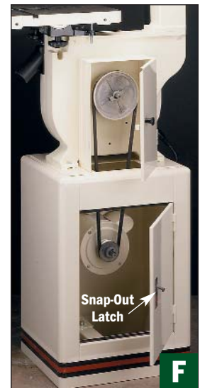
▶ The Jet makes it easy to service the entire saw by hinging every cabinet door.
