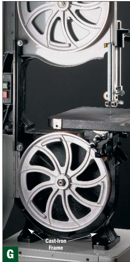
▲ Cast-iron frames have less resaw capacity out of the box, but can be expanded. The heavier nine-spoke wheels help dampen vibration.
