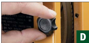
▲ Threaded knobs like those on the Powermatic make it inconvenient to open the wheel covers.
