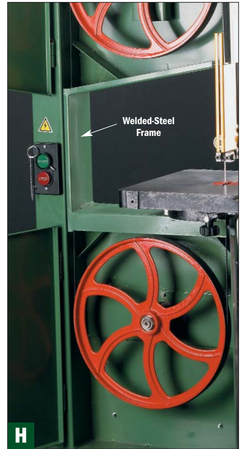
▲ Welded frames start with greater resaw capacity, but are not expandable. The lighter six-spoke wheels absorb less vibration.
