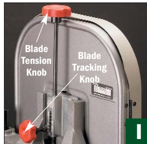
◀ Ridgid's large rubberized knobs make tuning the saw painless.
