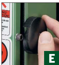
◀ The cam-lock knobs on the General lock the covers firmly, but still provide easy access.
