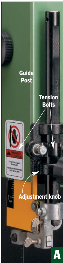
▲ General's tensioned guidepost operates smoothly.
