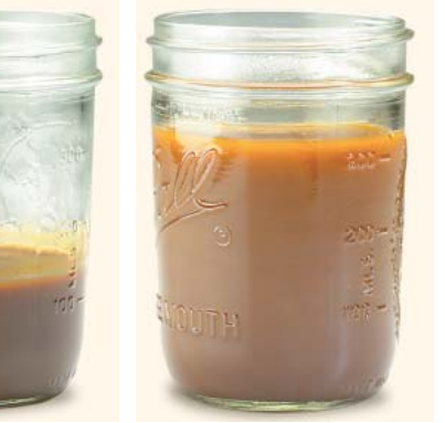
▲ The jar of shellac on the right is thinned with two parts denatured alcohol. The color is lighter and it will "flow" much better.
